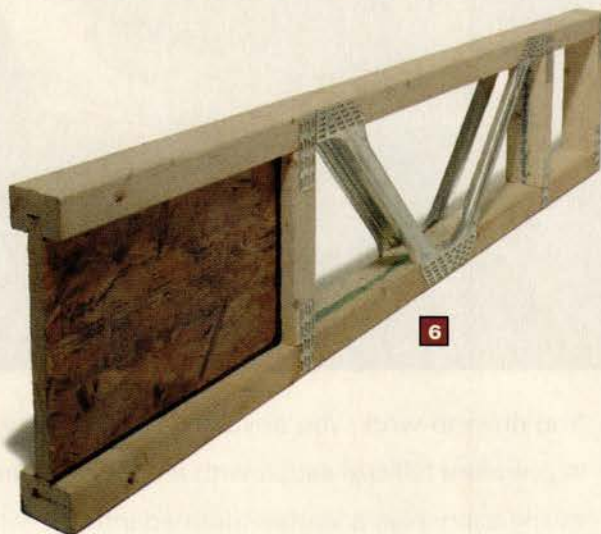
6. The open-web truss is steel-and-lumber hybrid that easily allows wires, ducts, and pipes to be snaked through. Although more expensive to make, its strength is comparable to similar-sized but much heavier steel beams.
