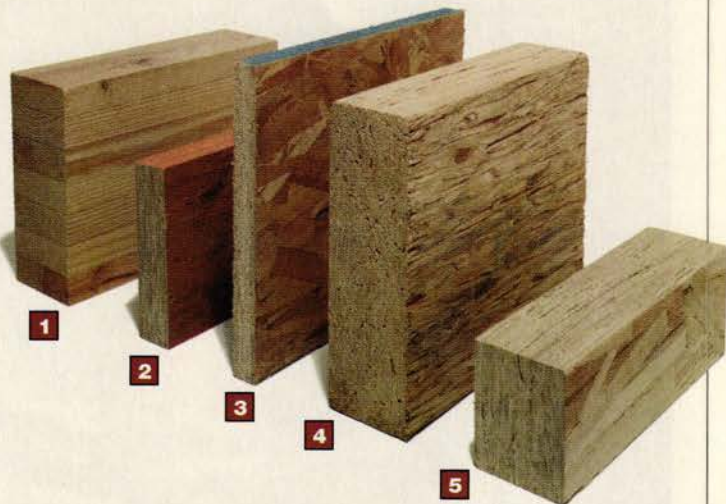
1. Glue-laminated (glulam) beams have multiple layers of sawn timber bonded together, often in graceful curves. 2. Laminated veneer lumber (LVL) looks like plywood, except that all the veneers' grain runs parallel to the beam's length. 3. Oriented strand board (OSB) works fine on rim joists, which don't bear heavy loads. 4. Parallel strand lumber is made with wood slivers, heated and pressed into beams stronger than a glulam of the same size. 5. Laminated strand lumber, made of abundant aspen and poplar trees, is being turned into studs as well as headers.
