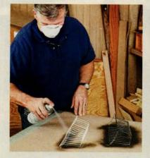
**6** Paint the wire baskets. While the rack dries, coat the wire baskets with spray primer and paint so that they match the coat hooks. Allow the paint to dry for at least two hours, then flip the baskets over and paint the other sides. Add a second coat of paint if desired.
