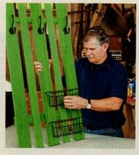
8 Hang the baskets and install the coatrack. Hold the baskets in place and mark positions for two cup hooks per basket. Screw the hooks into the 1×4s, and hang the baskets. Screw the other half of the French cleat to the wall, with its narrow face resting on the wall and its square edge facing down. Hang the coatrack on the wall-mounted cleat.
