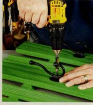
7\_Install the coat hooks. Attach one coat hook to each 1×4, using the screws provided. Position the hooks about 9 inches down from the top end of the coatrack, and be sure each one is centered on the 1×4.
