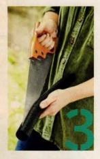
↑ Sheathe a saw. Slide a length of insulation over the blade of a handsaw to protect the teeth and your fingers when it's stored.
