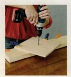
**LMAKE THE TRAYS** Cut 8-, 10-, and 111/2-inch squares from a 1/2-inch oak board. Drill 5/16-inch holes through the center of each tray, and glue
