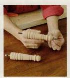
4\_INSERT SCREWS Unscrew the threaded bolts from the middle and top posts, and replace them with 5/16-inch dowel screws.
