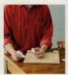
2\_ADD THE FEET Cut small squares of oak for feet. Apply a dab of superglue to the bottom corners of the base tray. and glue the feet in place.
