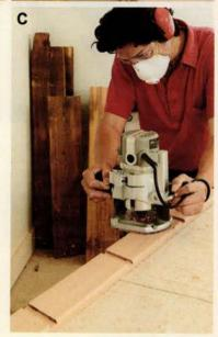
TIP Router bits spin clockwise, so for the greatest control, move the tool in the direction that keeps the bit biting into the wood.
