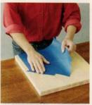
**L**POSITION THE TEMPLATE With a restickable glue stick, adhere the cut-out template to the butcher block.
