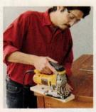
2 CUT THE SIDES Using a jigsaw, cut along the lines to form the tapered sides of the carrier.
