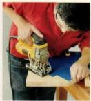
2\_MAKE LARGE CUTS Using a jigsaw fitted with an aggressivetooth blade, follow the template, stopping short at the corners.
