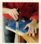
3\_TRIM THE CORNERS Use a fine-tooth pull saw to finish cutting the corners. Clean up rough-cut edges with a rasp, then sand.
