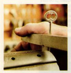
Reader-tested: Replacing a lost skeleton key just takes careful marking and filing.
