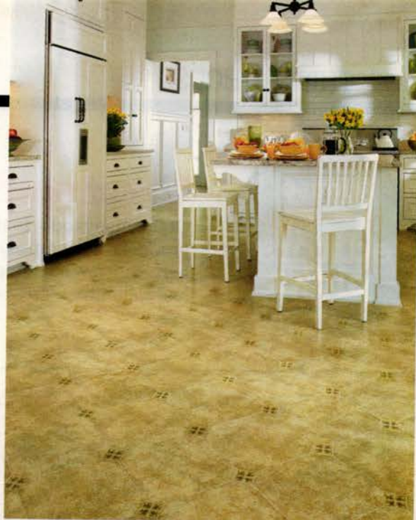
A sheet-vinyl floor can be placed over any surface, even tile, as long as it's smooth, flat, and dry.
