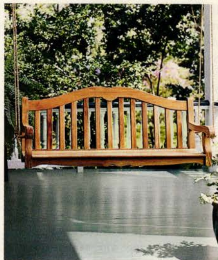
A friendly porch swing requires sturdy support: a 2x6 or larger ceiling joist and a hefty pair of 1/2-inch-diameter galvanized eye screws. To learn how to hang a swing, go to thisoldhouse.com/oct2015 .
