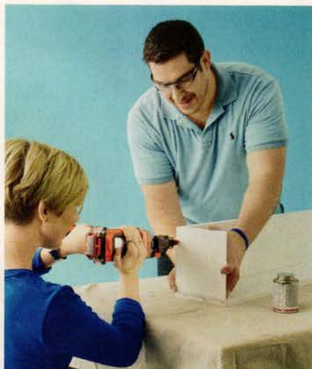
> Brad nails act as clamps to keep the PVC sides together while the cement cures.
