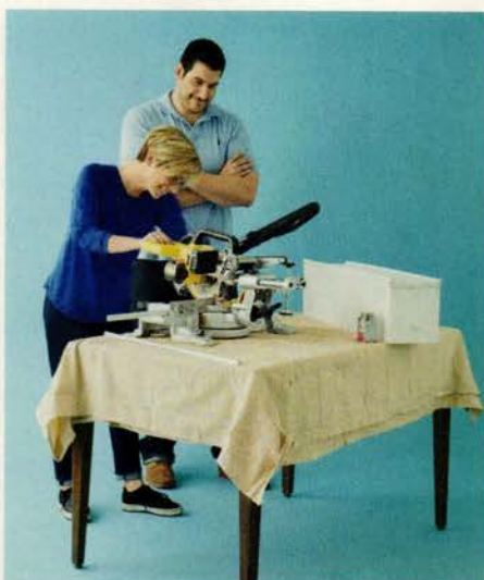
> Lengths of molding , cut with the miter saw, frame the top and bottom of the planter.
