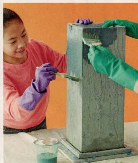
> Paint would have masked the wood-grain detail, so the team added color with a penetrating concrete dye. ■
