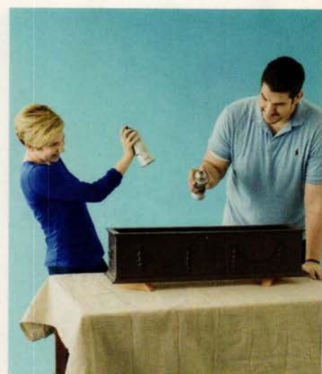
> When they weren't threatening to spray each other, the team coated the planter with black paint. A second coat, with a textured brown paint, gives the box a vintage, oxidized look.
