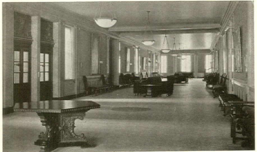
Upper Corridor, with Tennessee marble floor, inset with Levanto and Verte Tinos. The dado and pilasters are Botticino and the columns at each end are Gray Siena.
