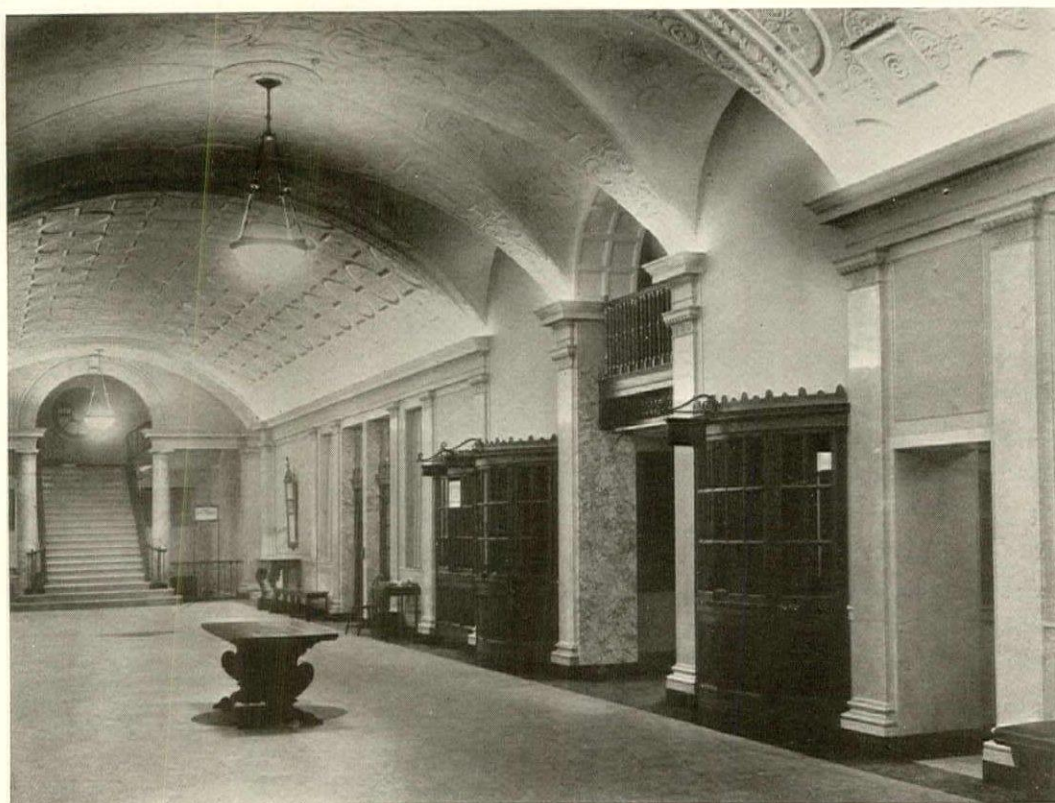
Main Corridor, with Tennessee marble floor bordered with Belgian Black. The walls are Botticino, with bases of Black and Gold.
