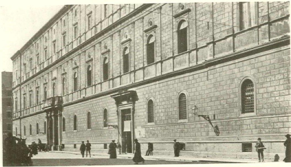
Exterior of the Palazzo della Cancelleria, Rome. The exterior is Roman Travertine stone, extensively used in Italy.
