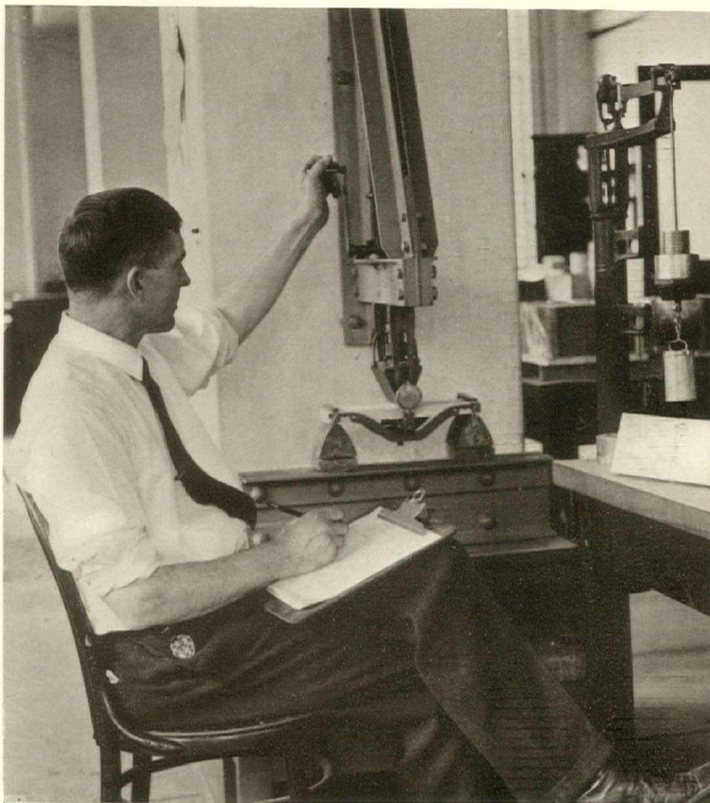
This machine, which measures the transverse strength and elasticity of marble slabs, is one of several pieces of apparatus devised by the United States Bureau of Standards in Washington and used in the Bureau's study of problems relating to the marble industry. Mr. D. W. Kessler, the author of the foregoing article, who is in charge of this research work, is shown operating the handle of the machine.
