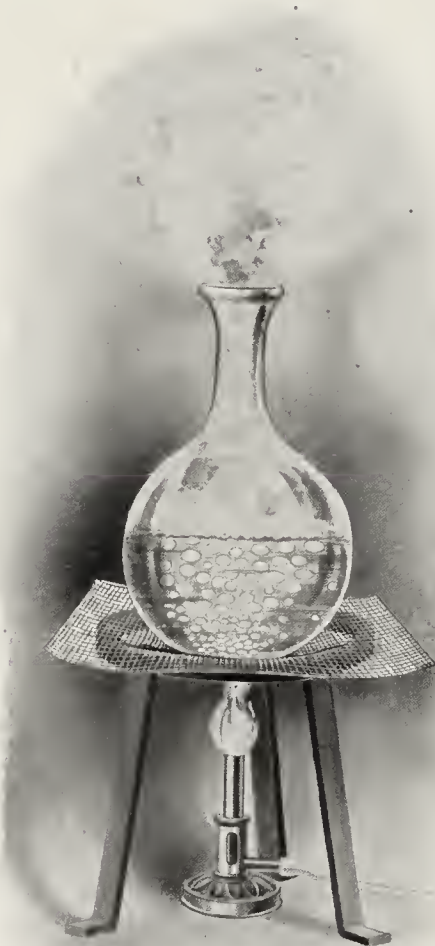
Water boiling under ordinary conditions—Temperature 212° F. or 100 C. Pressure 14.7 lbs. or 760 mm.
