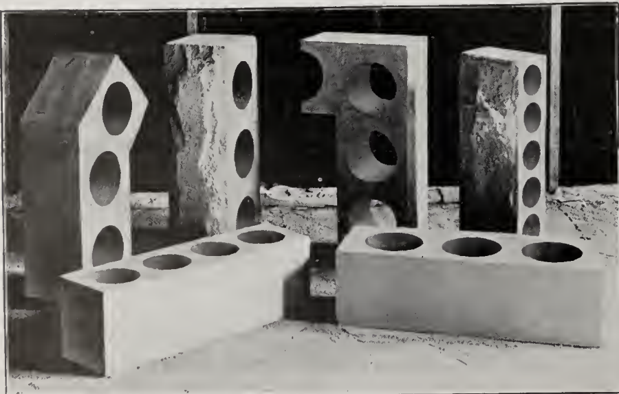
SPECIMENS SHOWING HOLLOW BUILDING BLOCKS.
