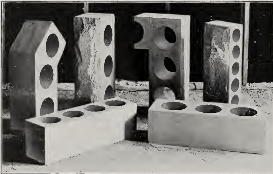
SPECIMENS SHOWING HOLLOW BUILDING BLOCKS.
