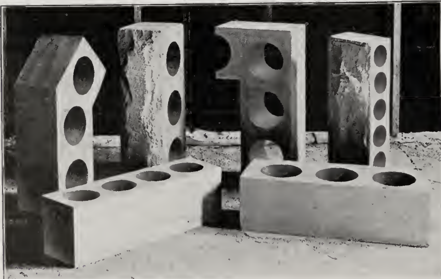
SPECIMENS SHOWING HOLLOW BUILDING BLOCKS.
