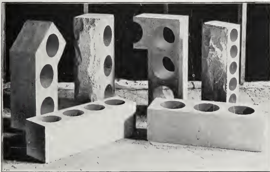
SPECIMENS SHOWING HOLLOW BUILDING BLOCKS.
