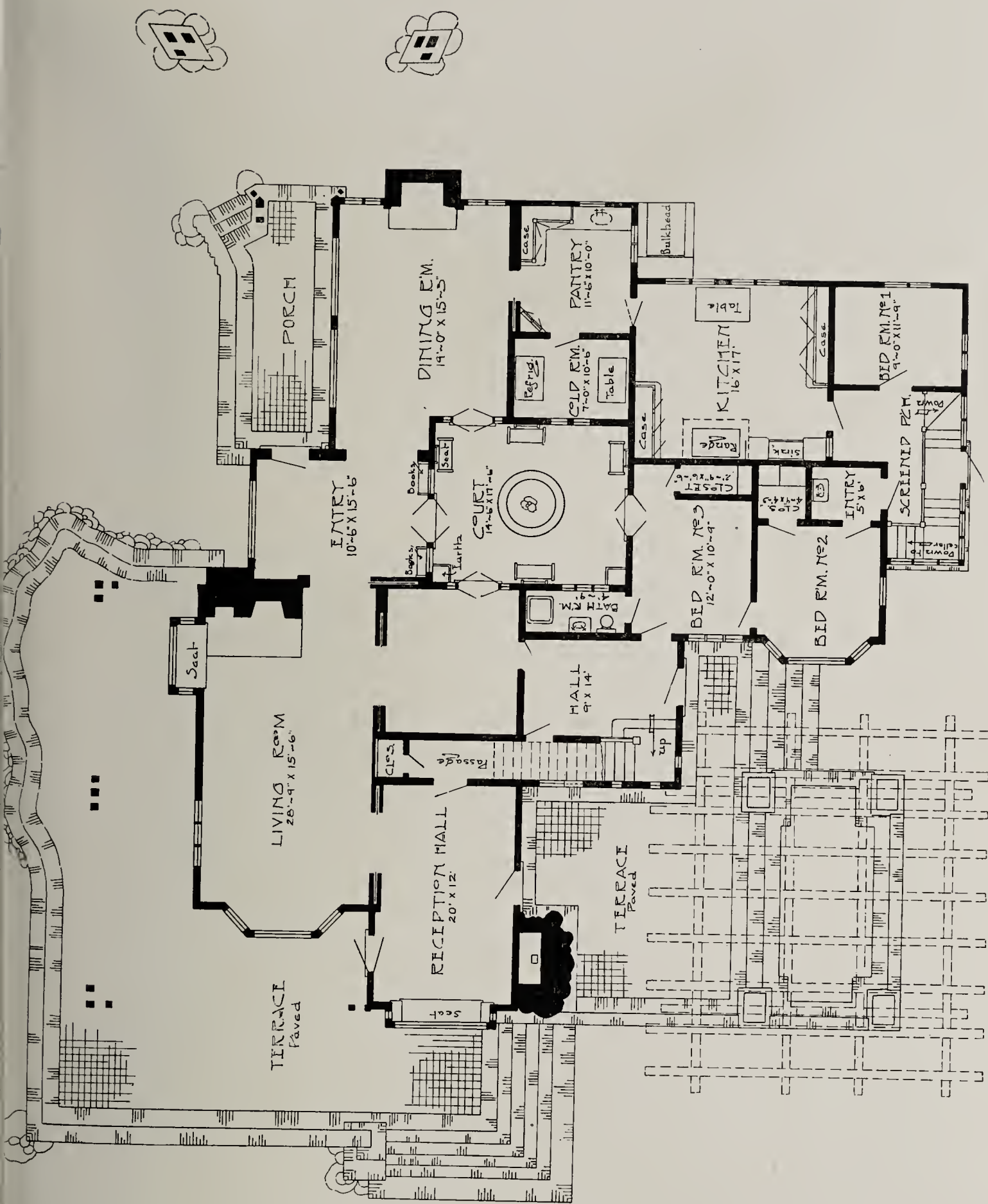
FIRST FLOOR PLAN PLANS OF BUNGALOW NUMBER 6 GREENE AND GREENE, ARCHITECTS, LOS ANGELES, CALIFORNIA
