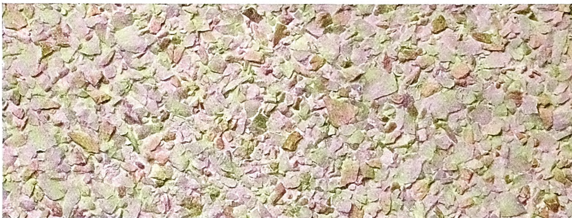
Hunt House formula: 1 part Atlas-White Cement; 1 part white quartz and pink felspar dust. While plastic, 1 part quartz and 3 parts felspar, \frac{1}{4} -inch grits thrown on and lightly floated.
