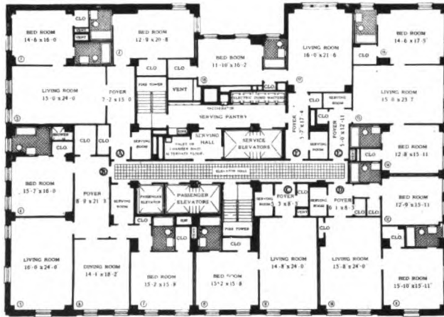
TYPICAL FLOOR PLAN, RITZ TOWER, SIXTH TO EIGHTEENTH FLOORS. EMERY ROTH, ARCHITECT.
