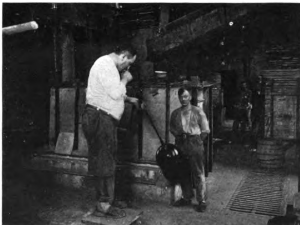
FIG. 2. BLOWING OF THE MOSAIC GLASS.
