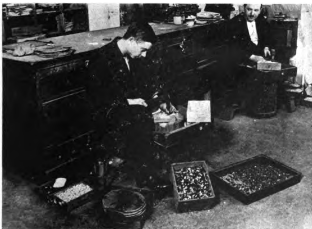
FIG. 1. CUTTING THE MOSAIC GLASS.
