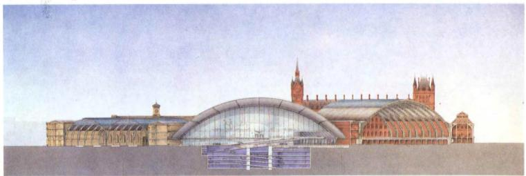
North-south section through Foster's terminal building bridging the gap between the Victorian buildings.
