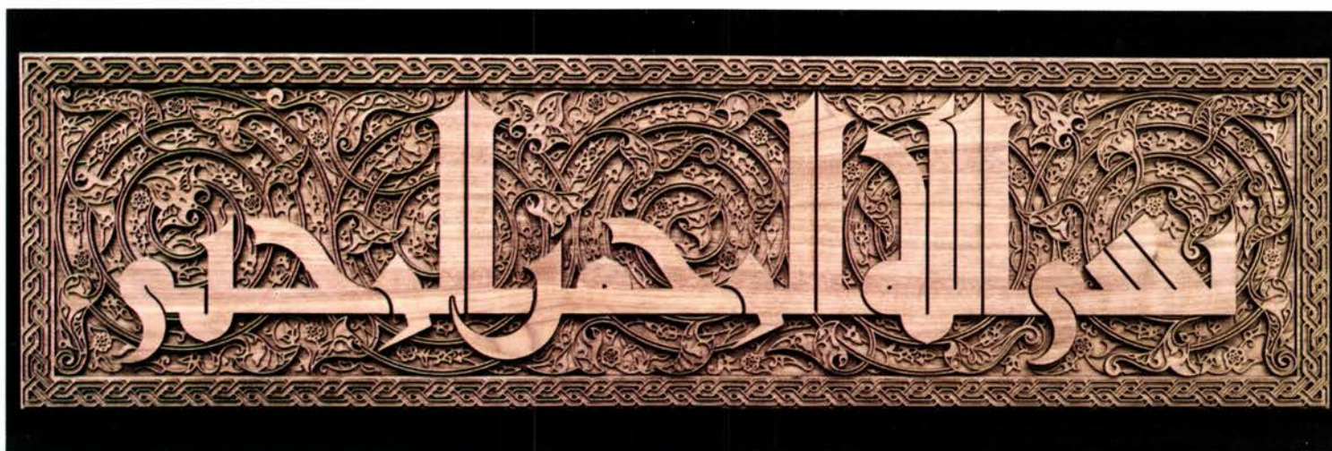
Laser-cut wood panel in Mamlouk style. Kufic calligraphy and floral background in 4 levels. Designed and implemented using CAD/CAM.
