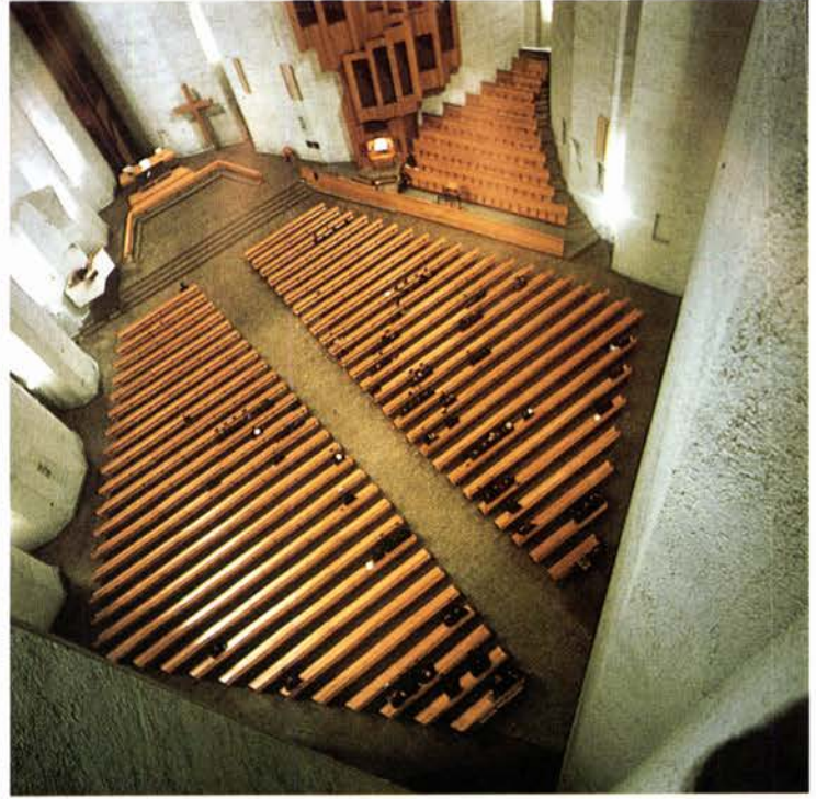
Exposed concrete wall interior with light yellow tiles on the exterior. Vertical window elements of thermoglass with wooden sashes. Trim and furniture are of pine, with a sand brown clinker forming the floor.
