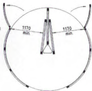
The Free-Flow system almost doubles the capacity, for use in panic situations.
