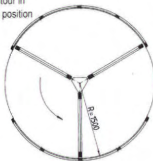
Once the doors have been unbolted, they can be folded together.
