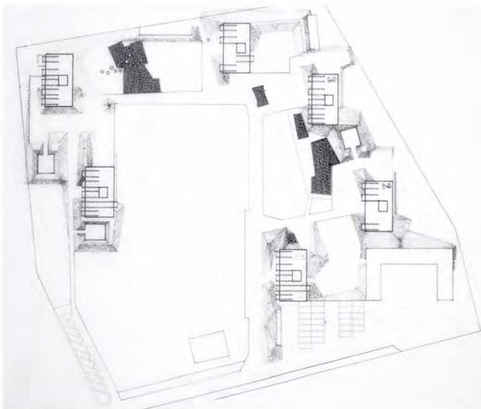
Sketch of an idea and (right) plan for the housing area at Lassaskog, Växjö. Balconies are suspended from the roof. Cold conduction is thus avoided, as floor elements do not project out into the cold as balcony floors.
