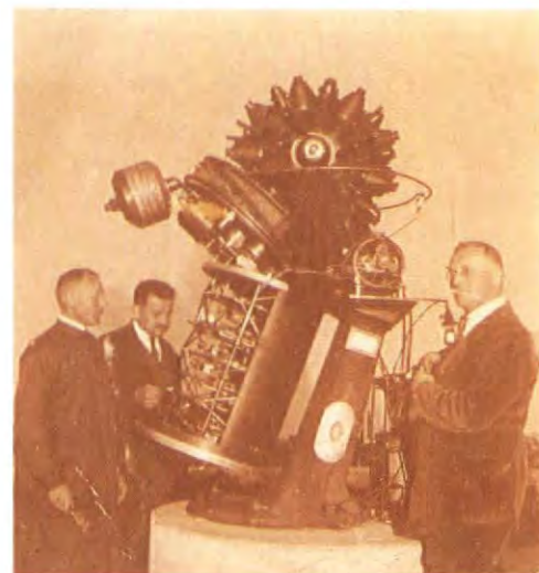
(Above left) Patented projecting machine; the geodesic divided sphere provides light beams for fixed stars, the cylinder contains moving spot lamps for the planets.
