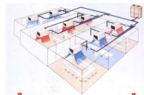
Ideal for both new build and retrofit, the advanced Daikin VRV head recovery air conditioning system (below) provides cooling and heating simultaneously from eight indoor fan coil units on the same refrigeration circuit. Circle #79.
