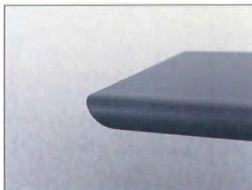
Ends of desktops are neatly finished by using matching laminate on the underside formed upwards on a large radius. The resultant corner detail accentuates and compliments the overall design.
