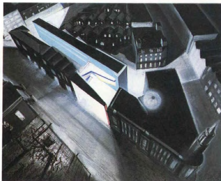
Grand Buildings competition entry, Trafalgar Square. The building comprises two parts: a stone slab which forms a service and access backbone to the site, and a curved block with a glass skin, which contains office spaces
