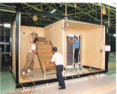
The Toyota Kasugai factory (left) with modular assembly unit (above)
