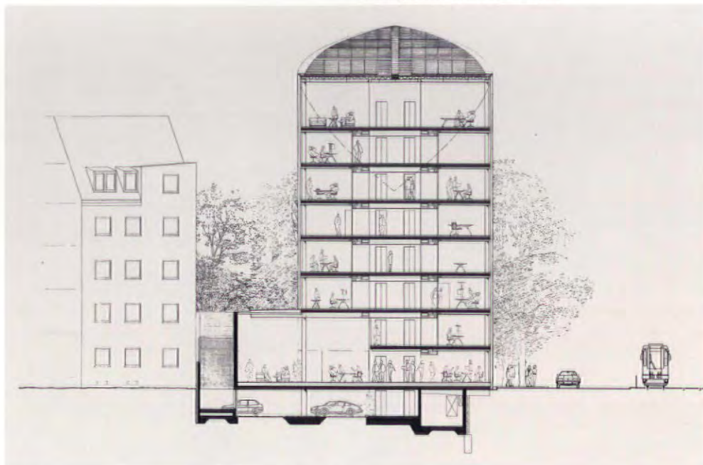
Cross section and long section (below) show general arrangement of accommodation
