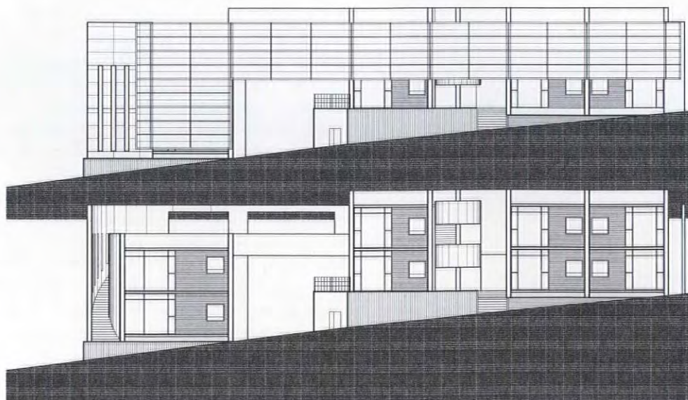
Top A semi-transparent wall protects the apartment block from the street creating a richly textured, three-dimensional facade. Above Site plan. Left Front elevation and section
