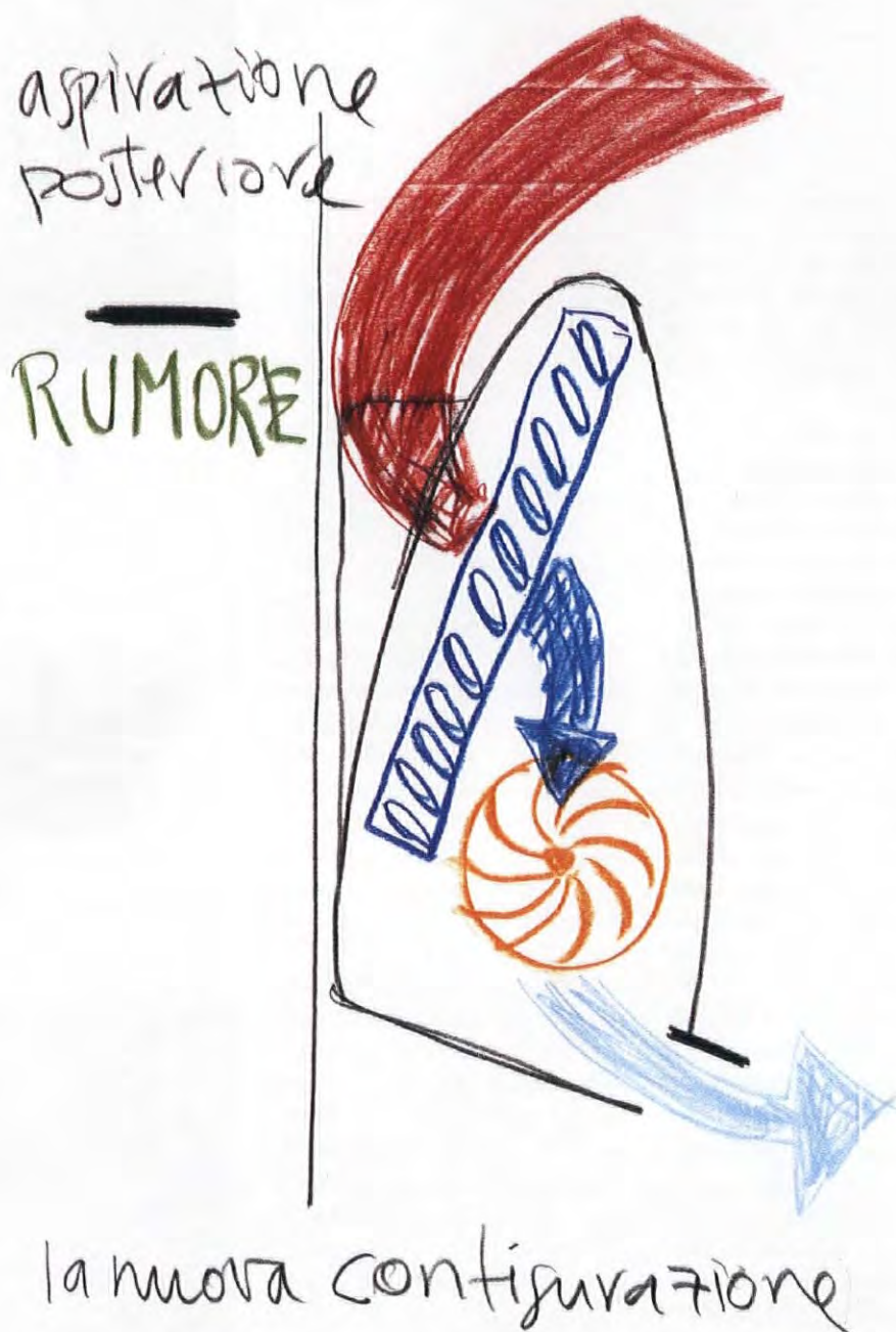
Above Design sketch of Clima Più, demonstrating the system's modifications to the traditional air-conditioning configuration.
