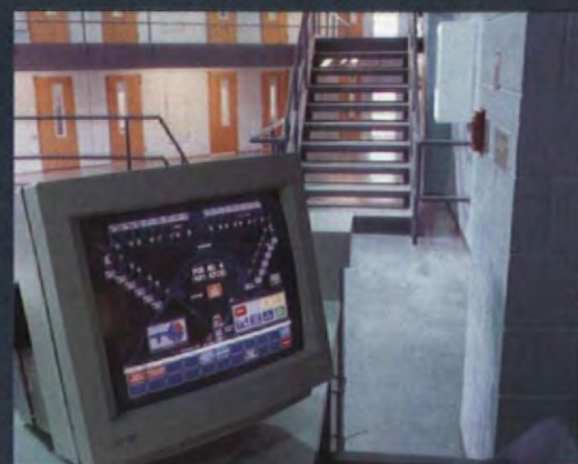
Touch-screen technology can be used to control the security of an entire prison from a central terminal
