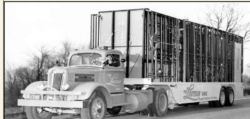
An official Lustron truck, specially commissioned by the Lustron Corporation and packed at the factory in the order needed at the building site.
